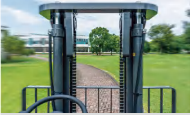
Wide-view mast improves safety in stacking operations.
