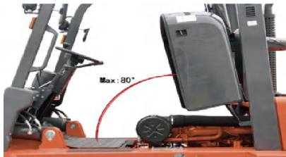
The hood opening angle is increased to 80°, making maintenance more convenient.
